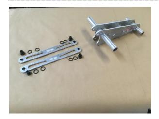
We designed a pull rod set which works with the aluminum arm to make the suspension geometry progressive, providing increased comfort in small bumps while resisting bottoming. The progressive kit works particularly well with the ACT spring shock, or with the torsion spring kit.
